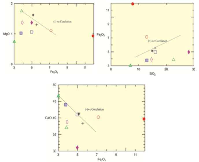
Fig.6 : Shows Mutual Relationship between Fe<sub>2</sub>O<sub>3</sub>Vs MgO,CaO and SiO<sub>2</sub>Vs Fe<sub>2</sub>O<sub>3</sub>
