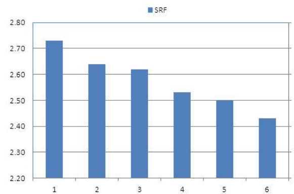
Fig. 17. The diagram shows the values of SRF for six models of joint on the slope with dip of 75 degrees (1-Parallel deterministic, 2-Parallel statistical, 3-Cross jointed, 4-Baecher, 5-Veneziano, 6-Voronoi)
