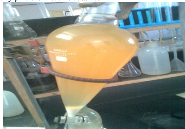
Fig 3.4 Removal of Catalyst
