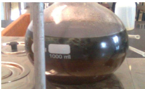
Fig 3.1 Reaction of Vegetable oil and Methano
