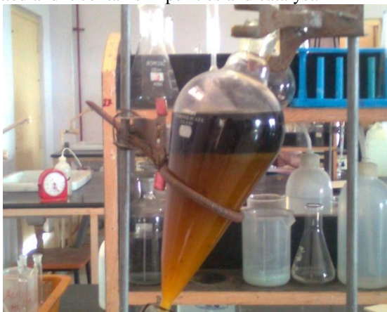
Fig 3.2 Separation of Bio-diesel and impurities of Honge oil
