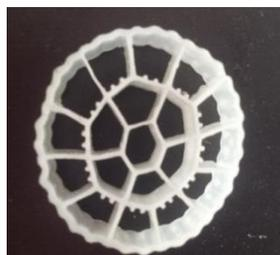
**Figure 3:** Media added into the reactor 1
